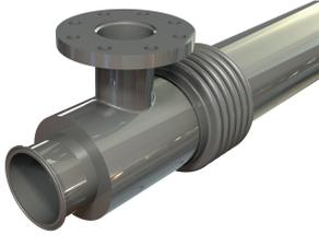
The HRS DTA Series is a complete stainless steel double tube heat exchanger designed for hygienic applications. The product flows through the inner tubes and the service fluid flows through the surrounding shell. As a result of its geometry, the DTA Series has a continuous free-pass cross section allowing large particles to be processed and reduces the risk of product blockages.
