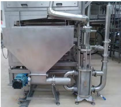
The HRS BPSC Series is specifically designed for highly viscous materials such as pastes and particularly those which are produced and packed at low temperature.
