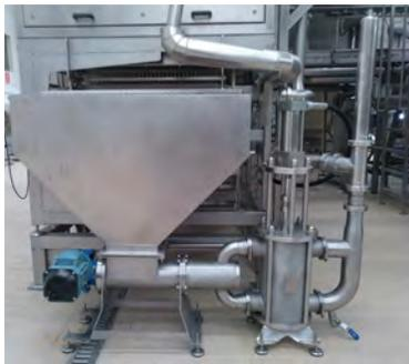
The HRS BPSC Series is specifically designed for highly viscous materials such as pastes and particularly those which are produced and packed at low temperature.
