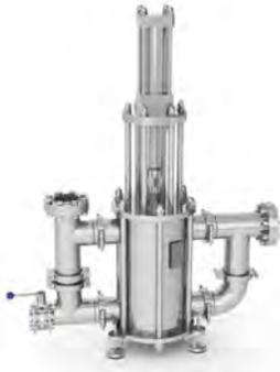
The HRS BP Series piston pump is a fully hygienic, hydraulically operated positive displacement pump. The pump is driven by a hydraulic power pack which drives a hydraulic cylinder from alternate directions, moving the piston up and down.
