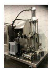
The BPM Series is a mobile version of the standard BP Series pump. It is mounted on a mobile skid unit for easy movement, allowing it to be used across multiple production lines and locations, ideal for food manufacturers producing short runs of specialist products.
