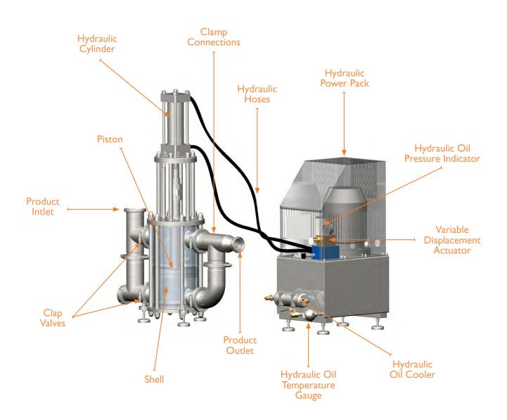
BP Series pumps are driven by a hydraulic power pack which drives a cylinder in alternate directions, moving the piston up and down.
