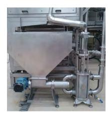
The HRS BPSC Series is specifically designed for highly viscous materials such as pastes and particularly those which are produced and packed at low temperature.
