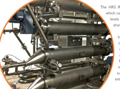
The HRS R Series technology uses a rotary scraper bar, which can reach speeds of up to 300rpm resulting in high levels of shear and mixing at the heat transfer surface; dramatically increasing the heat transfer rate.
