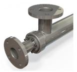
The HRS DTIR Series is a complete stainless steel double tube heat exchanger designed for industrial and environmental applications. The product flows through the inner tubes and the service fluid flows through the surrounding shell. As a result of its geometry, the DTIR Series has a continuous freepass cross section allowing large particles to be processed and reduces the risk of product blockages.
